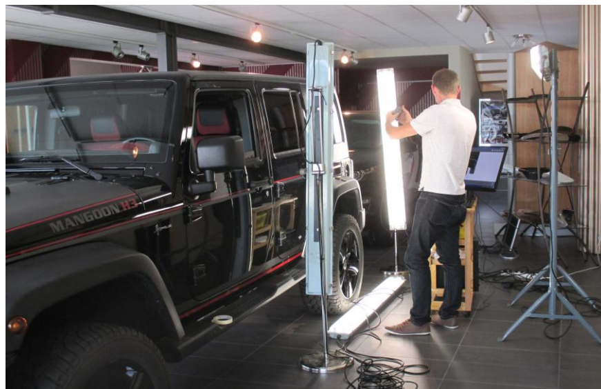
Next step: Scanning the car body to get base data for CAD engineering
